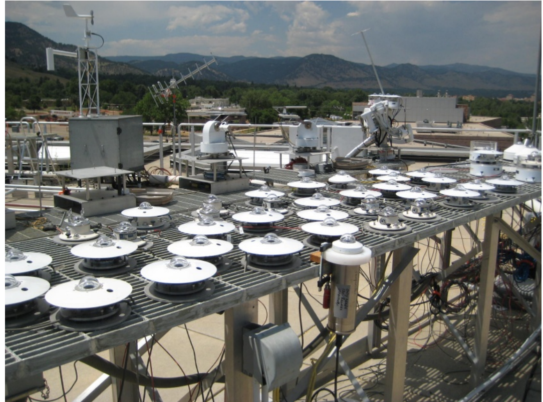
Rooftop radiative flux sensor calibration facility NOAA/ESRL/GMD Boulder, CO
